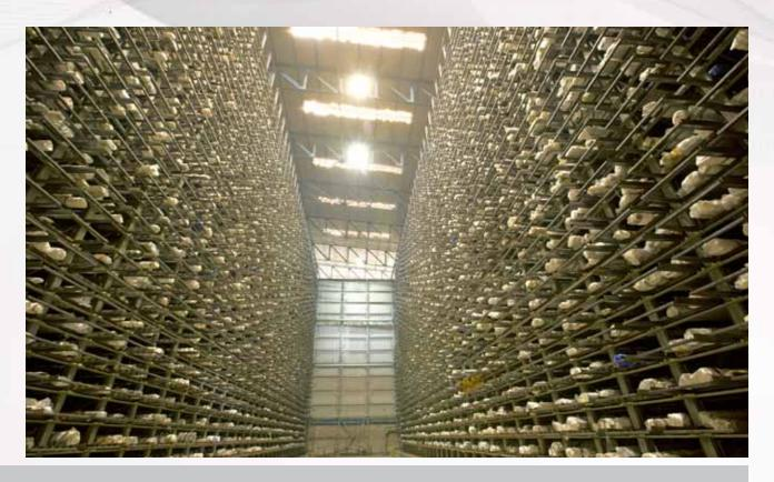
FeHR honeycomb warehousing system is completely suitable for large quantities and high access speeds. This system is used for automatic storage and retrieval of Bright Bars and Profiles. FeHR Cassette Rack System makes the best use of the available space and allows swift movement of the material from the packaging area to the storage area and all that is made possible with the touch of a button.
