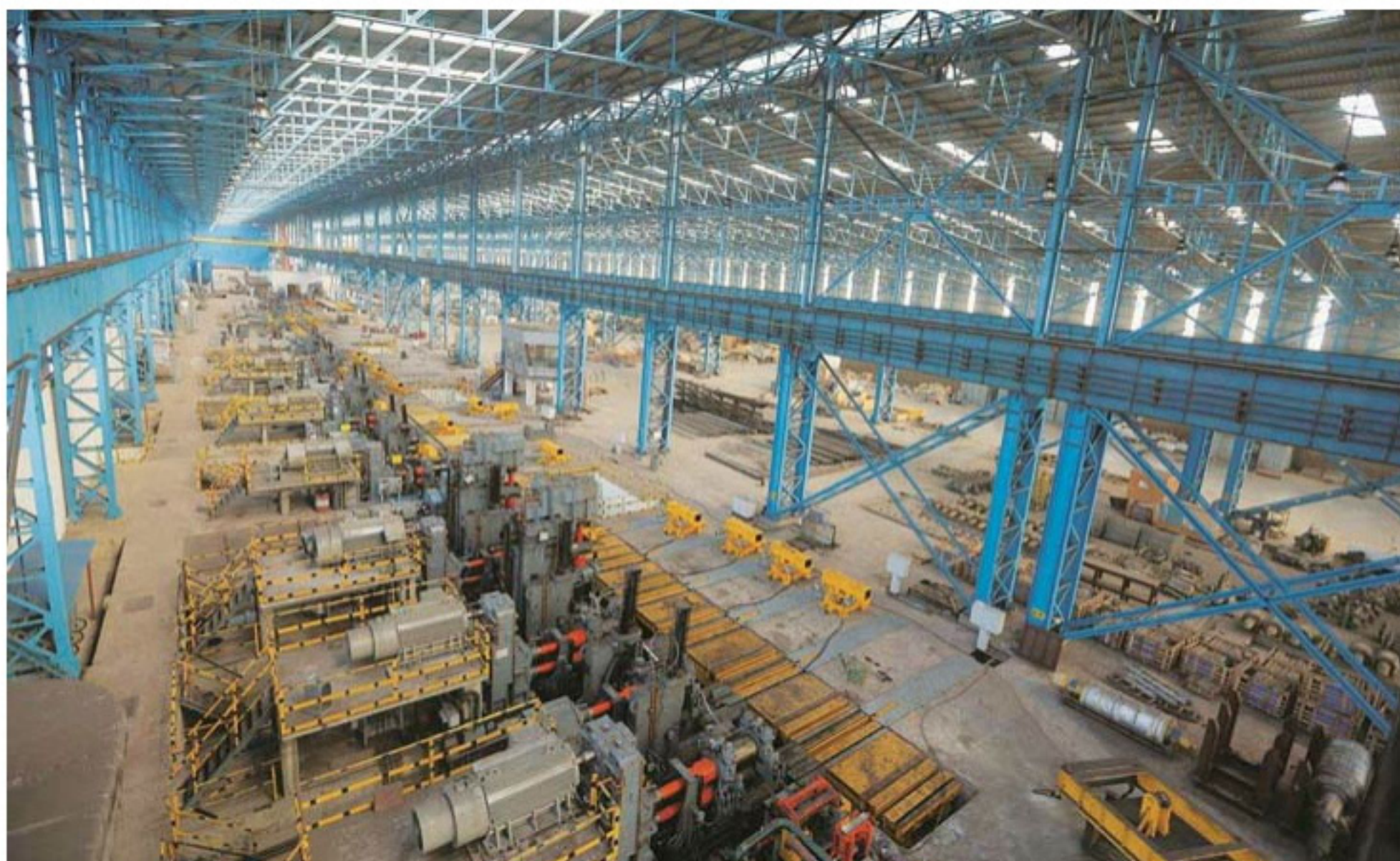
Viraj's new Section Rolling Mill (SRM) with an annual capacity of 180,000 tons p/a enables them to manufacture over 700 different shapes and designs of angle, flats and other profiles. Photo ©Viraj
