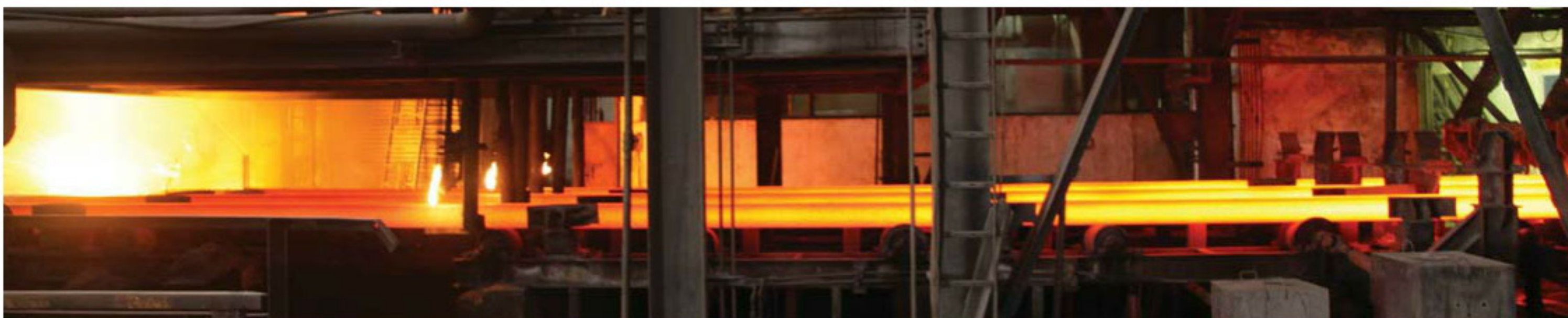
Continuous billet casting machine in use. Photo ©Viraj
