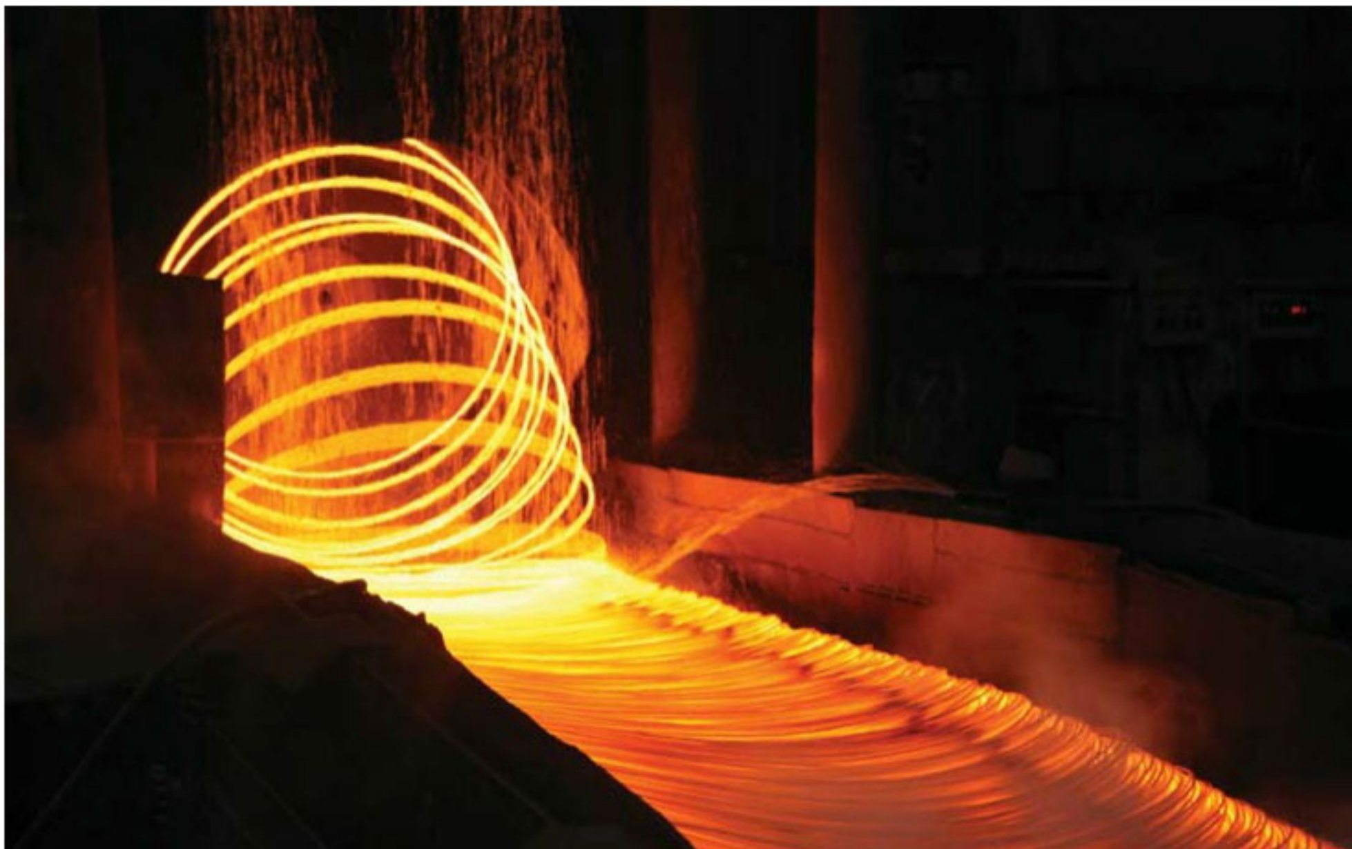
Wire rod mill in operation. Photo ©Viraj
