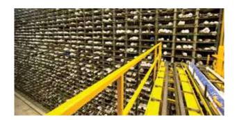
The installed capacity is of around 10,000MT. This system allows to optimize the warehouse space and our inventory management system. The minimum approach dimensions of the storage and retrieval units also create benefits and provide lot of flexibility in terms of storing and retrieval of the material.
